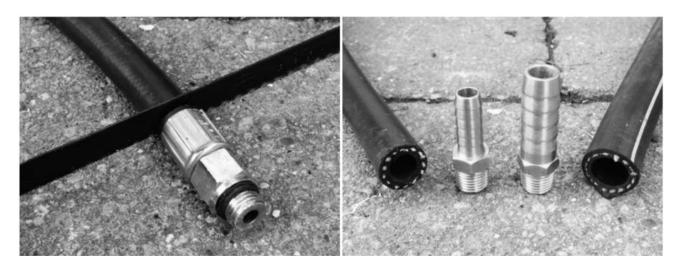
INSERT THE TAIL END INTO THE HOSE AND FASTEN A HOSE CLIP IN THE SAME WAY AS 7. (D).
