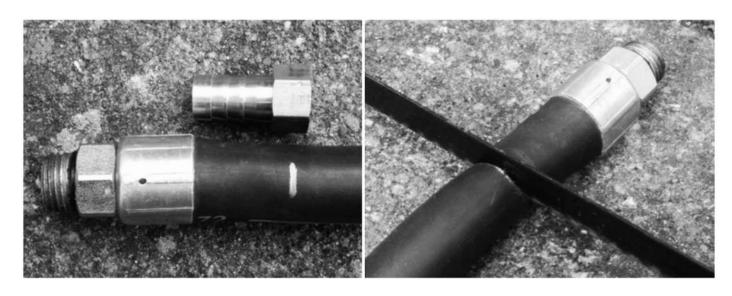
CHECK THAT THE HOSE TAIL END CONNECTOR IS A SNUG FIT INSIDE THE HOSE. IF NOT, SELECT A DIFFERENT DIAMETER.
