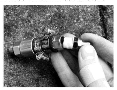
WITH AN ADJUSTABLE SPANNER TIGHTEN THE HEX BUSH FURTHER. YOU MAY NEED A SECOND ADJUSTABLE SPANNER TO HOLD THE HEX NUT ON THE HOSE TAIL END CONNECTOR.
