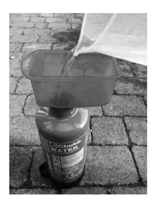
FIRST TRY WATER TO TEST YOUR MODIFICATIONS. THEN FOR PAINT MIXTURES TRY 1 PART PAINT TO 1 PART WATER, OR
