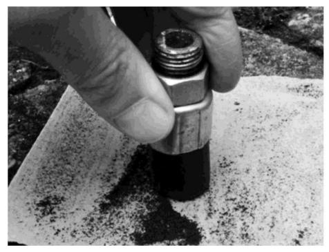
IF NECESSARY GRIND THE HOSE DOWN WITH SOME EMERY PAPER OR A RASP UNTIL THE BARB MEETS THE METAL CENTRE. BE CAREFUL NOT TO MAKE THE HOSE TOO SHORT.
