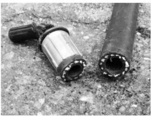
THE PROBLEM NOW IS THAT THE INSIDE OF THE HOSE WILL HAVE A LARGER INTERNAL DIAMETER THAN THE HOSE CONNECTOR, ESPECIALLY ON A JET SPRAY HOSE. WHETHER IT WILL STILL PRODUCE AN ACCEPTABLE JET DEPENDS ON HOW BIG THE DIFFERENCE IS — TEST IT. A BETTER OPTION IS TO MAKE A NEW NOZZLE (SEE NEXT SECTION).
