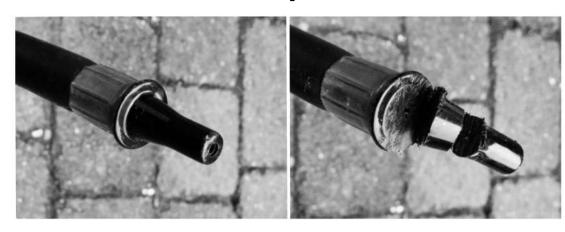
ANOTHER OPTION IS TO CUT THE NOZZLE OFF ENTIRELY, EXPOSING THE FULL INTERNAL DIAMETER OF THE HOSE.
