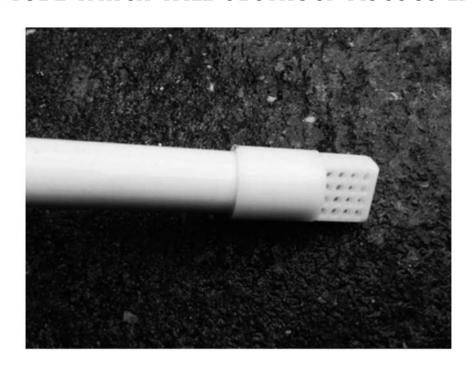
THE FILTER MIGHT UNSCREW, IF NOT, USE A HACKSAW TO CUT THE END OFF UNTIL THE FULL INTERNAL DIAMETER OF THE SYPHON TUBE IS EXPOSED. CUT AS NEAR TO THE END OF THE TUBE AS POSSIBLE TO AVOID SHORTENING IT.
